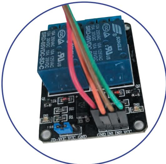
Here you can see the header wires on the relay board. Notice the cable colours and how they match the pins above.
