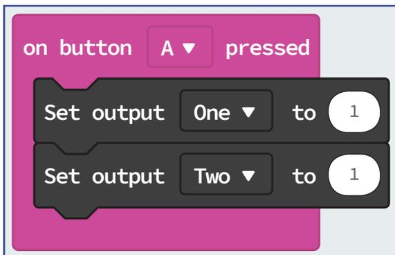
This simply sets each of the outputs to 1 (on) once button A is pressed.
