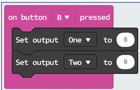
In this example we set the button B to set the outputs to 0 so that we can use it to turn of the robot drone.
