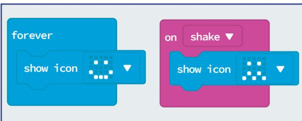
A simple interaction to start with is the micro:pet reacting to being shaken. Here, the micro:bit's accelerometer senses when it is being shaken using the *on shake* block. It then shows a sad face to represent the micro:pet being unhappy when it is shaken.
