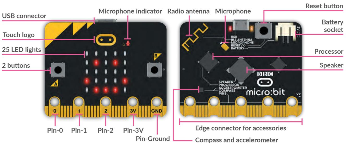
The most obvious way to tell which micro:bit version you have is by looking at the pins. The new micro:bit has notches that help keep crocodile clips attached and prevent them touching the other pins by accident when moved.
