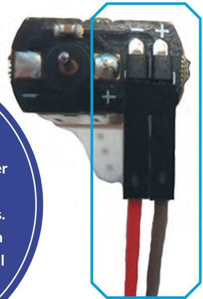
Here you can see how the servo motors are wired to the servo controller and micro:bit.
