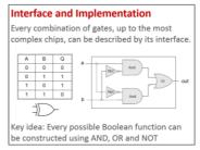
Any chip can be decomposed down to individual AND, OR and NOT components. There is no better example of the relationship between decomposition and abstraction than chip design. Once constructed, the detail of the implementation can be abstracted away. The circuit designers can focus on connecting interfaces, without worrying about the detail of implementation.
