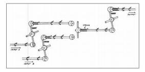
Diagrams demonstrate how we could fashion an OR and a NOT function using simple mechanical components. They come from a wonderful book "The Pattern On The Stone" by Danny Hillis (see further reading). Ask students to develop a truth table for the combinational logic circuit, constructed from 3 NOT gates and an OR gate. Point out that it performs as an AND gate. Only when both inputs are pushed (on), will the output also move forward.
