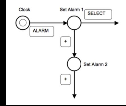
Working out the finite state machine of an alarm clock
