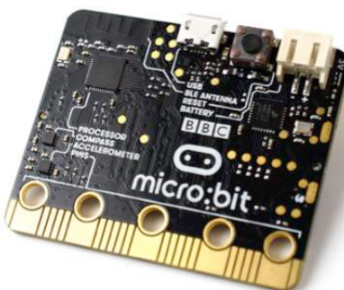
Figure 3.34 The other side of the BBC micro:bit showing power and data connectors, processor, accelerometer, compass and reset button
