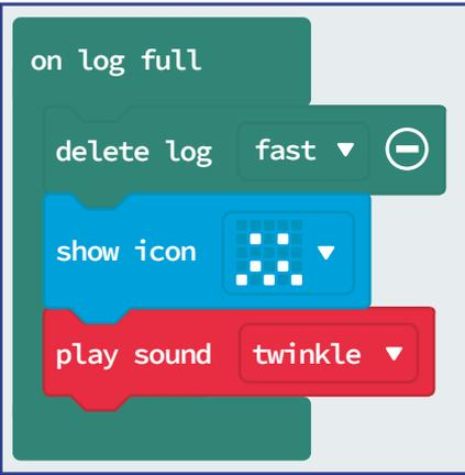
Now let's add the blocks that allow the micro:bit to keep recording even once the memory is full. These blocks tell the micro:bit to overwrite the oldest data with new data.
