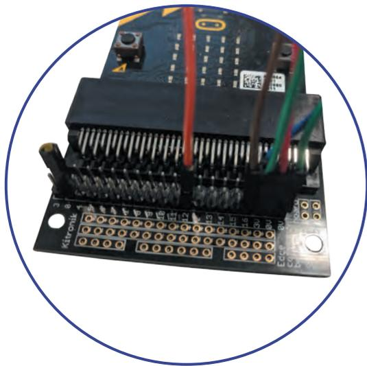
In this image you can see how the micro:bit breakout edge connector is used to connect the header cables to the relay and the moisture sensor.
