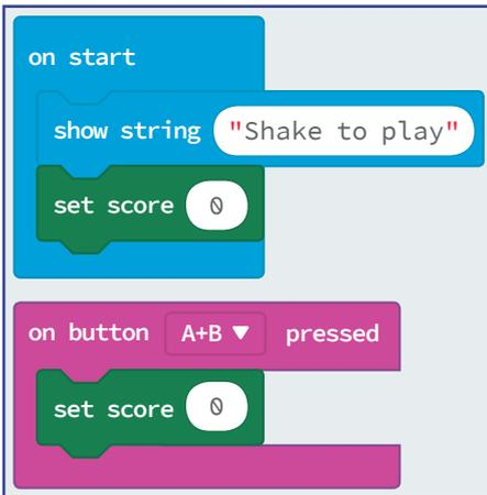
Here we create the initial user interface by telling the user to “Shake to play”. Then we use the **set score** block (in the ‘Game’ blocks menu) to set the score to 0 when the program first runs and also when **A+B** are pressed.
