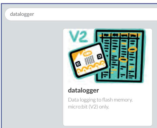
Type “datalogger” into the search box and you should see the new datalogger extension. Notice that “datalogger” has no spaces—you will get many more results if you type “data logger”.
