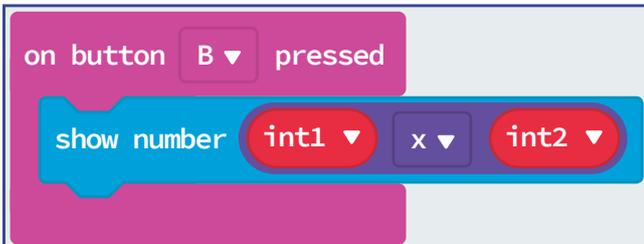
Again we use an *on button pressed* block but this time for button B and we also add the *show number* block. Inside that block we use another *Math* block to multiply *int1* with *int2*.
