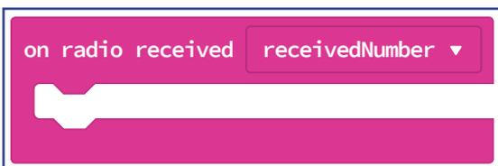
This block receives the radio signal from the other micro:bit and stores the number in a variable called **receivedNumber**
