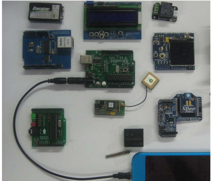
Since the files for it are Open Source lots of compatible boards are available. It's designed to have sub-systems called shields stacked on top of it: in the photograph above clockwise from top left are some examples: Ethernet, LCD screen, relays, colour graphics screen, XBee wireless transmitter/receiver, GPS system and aerial, RFID reader (and small glass tag), solar panel and battery (connected to an Arduino) as an alternative power source, and an Arduino to composite TV shield!
